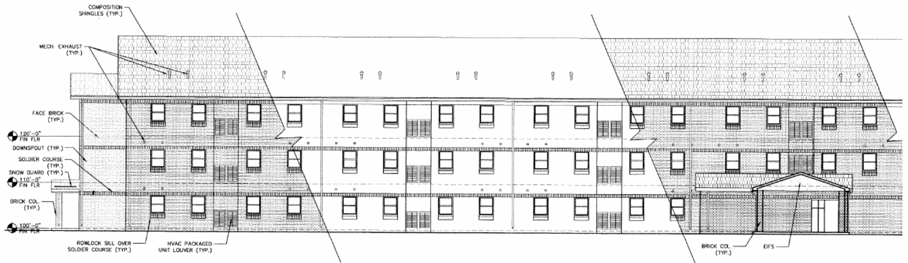
A FRONT ELEVATION 0' 4' 8' 12' 1/8" = 1'-0"
